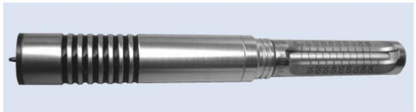
Typical indentation shore hardness gauge for field use.
