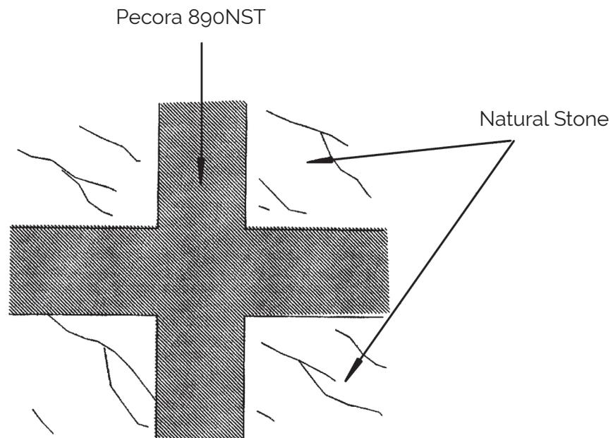
Sealant should be applied in a continuous operation using sufficient pressure to fill the joint and make complete contact to the joint sides. Tool the sealant slightly concave using solvent or dry-tooling techniques. Contact Technical Services prior to tooling with solvent. Do not tool with soap or detergent and water solutions.
