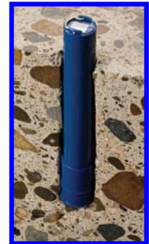
If the concrete is at 5.0% moisture content, it will neither absorb nor desorb moisture if the air above it is 70° F (21° C) and 75 percent RH. Therefore, if the air inside the box measures less than 75 percent, it can be assumed that the moisture content of the concrete is less than 5 percent
